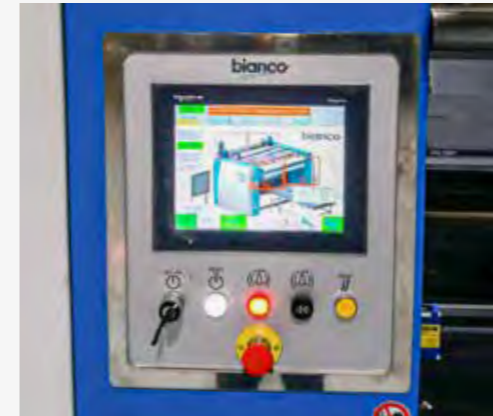
Touch screen panel Pannello operatore touch
