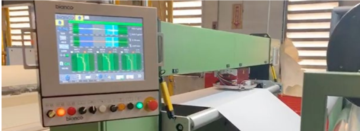
BIANCO traversing with Thickness detector STHA1 placed in a line to detect the thickness profile of a coated material
