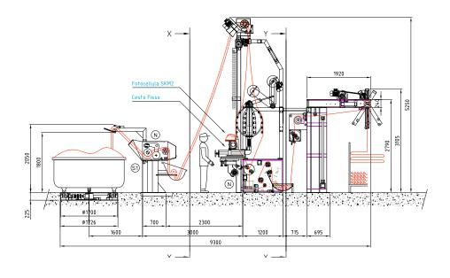
Bianco® Rope Opener & **Slitting line Tensionless** with accumulation scay
