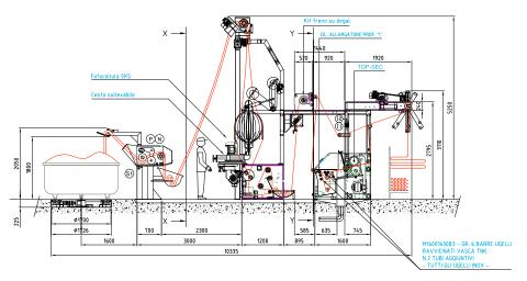
Bianco® Rope Opener & **Slitting line Tensionless** with accumulation scay, TNK and padder
